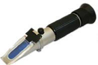
Easy – use a Kamco 402 Refractometer. This simple device can quickly tell you the percentage of anti-freeze in solution and whether the anti-freeze is propylene or ethylene glycol based. Not only that, but it will also tell you the likely degree of low temperature protection that you have.
