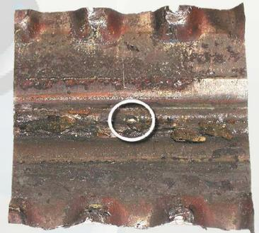
Corroded radiator showing pinhole
